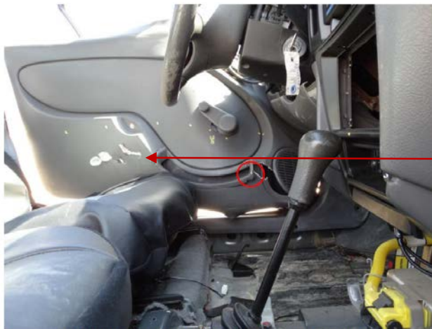
Figure 3.82: Location of Maximum Interior Deformation
