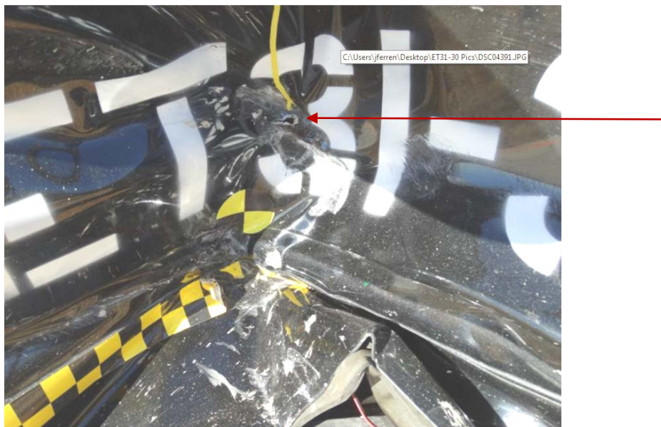
Figure 3.67: Post Test Vehicle – Left Side Door, Close-up
